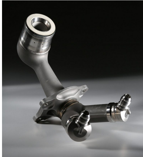
Figure 1. GE Aviation's 3D-printed fuel nozzle tip. [14]
